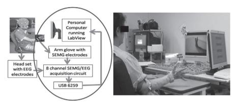
Fig.1. Block diagram of Rehabilitation Platform setup showing SEMG glove and Signal flow path
